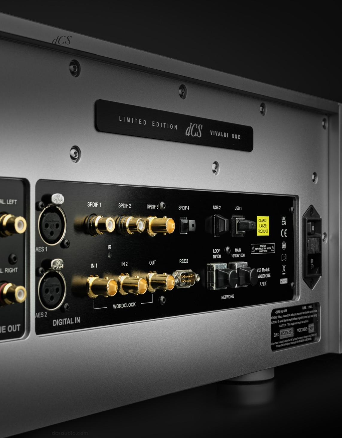
An array of digital inputs, plus multi-stage DXD oversampling with optional DSD/64 or DSD/128 upsampling, and user-selectable DSP and DSD filters, offer unrivalled flexibility. The system's performance is driven by flexible firmware, which can be easily updated to deliver new product features and enhancements.
